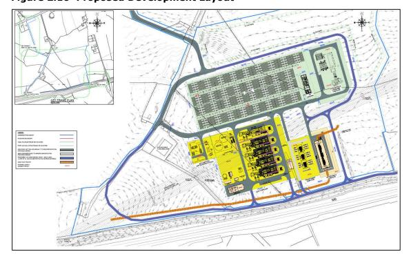
Connection of the LEL GIS Castlelost Project to the existing transmission system involved consideration of numerous layout options. These included (i) new in-line towers and transition from overhead line (OHL) to an underground cable (UGC) routing to the GIS
