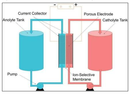
Figure 2.5 Vanadium Redox Flow Battery
