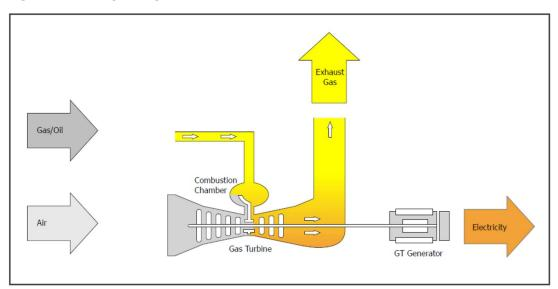
OCGT units are advantageous due to their operational flexibility and can be turned on quickly to provide peak load. The LEL Flexgen Castlelost reserve generator is designed to get to full load in less than 10 minutes. OCGTs exhaust residual heat to atmosphere at a temperature of approximately 544°C, i.e., unlike combined cycle gas turbines (CCGTs) where exhausted heat is recycled to generate steam and ultimately additional electricity. The OCGT units have a typical energy efficiency of 38-41%.
